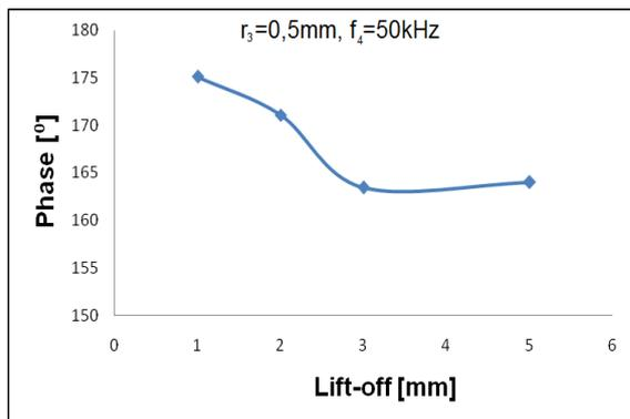
Fig.12: Dependence of maximum impedance phase on lift-off
