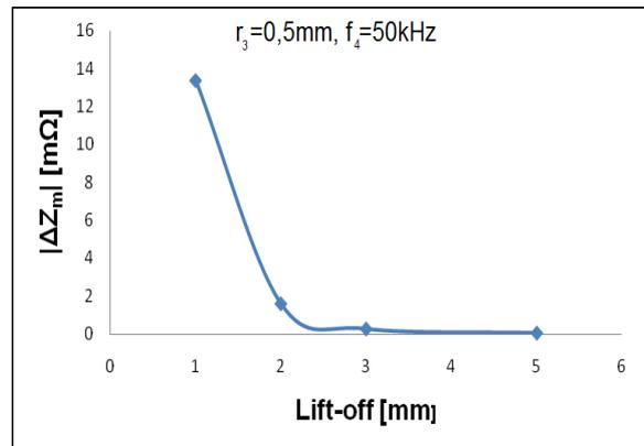
Fig.11: Dependence of maximum impedance module on lift-off
