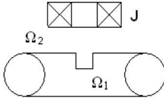
Fig.4: Typical configuration of ECT
