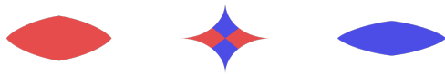
Figure 2: The glyph’s shape indicates the relation of both eigenvalue signs. A red glyph has two positive, the blue one two negative eigenvalues. They are therefore convex shapes. If the eigenvalues have opposite eigenvalues, the shape is concave.
