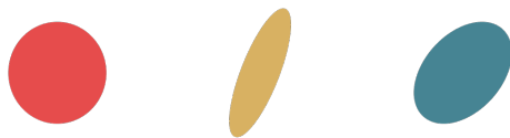
Figure 3: Ellipses indicate identical and/or complex eigenvalues. A perfect sphere indicates two identical eigenvalues, whereas ellipses represent rotational behavior. Colors close to yellow indicate counterclockwise, those close to green clockwise rotation.
