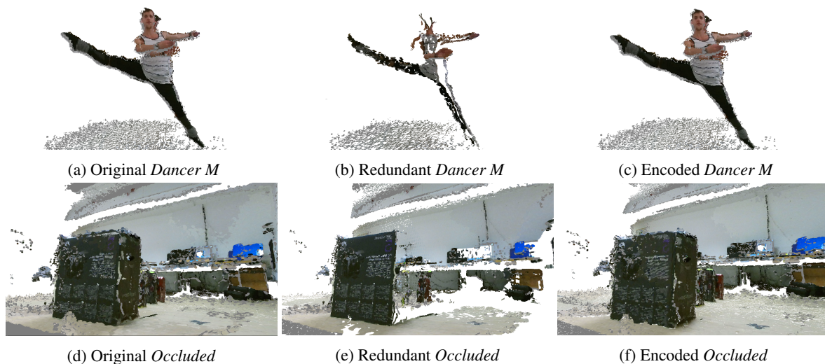
Figure 4: Result of the encoding process. Original (a, d), redundancy removed (b, e), and encoded data (c, f) for a wide and a narrow baseline scenario (top vs bottom row).
