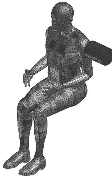
Fig. 5. Shoulder validation setup [1]
