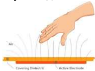
Fig. 3: Capacitive sensor's operation. [8]
