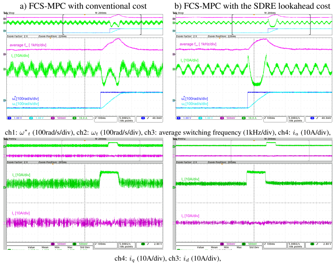
Figure 5.5.: Comparison of FCS-MPC with conventional cost (left) and with the SDRE lookahead cost (right) for step change of speed of PMSM drive from -100 to 100 rad/s at 6.25 Nm of load torque. Penalization \lambda_u was tuned to average switching frequency of 550Hz in steady state.
