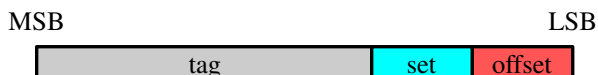
Figure 2: Address structure in relation to the CPU cache. The sizes of the individual parts depend on the particular architecture.
