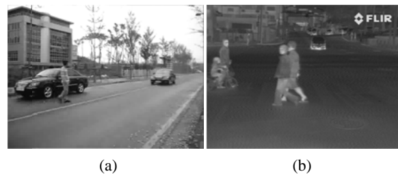
Figure 1. Sample images of pedestrians. (a) Visible spectrum image. (b) Far-infrared image.
