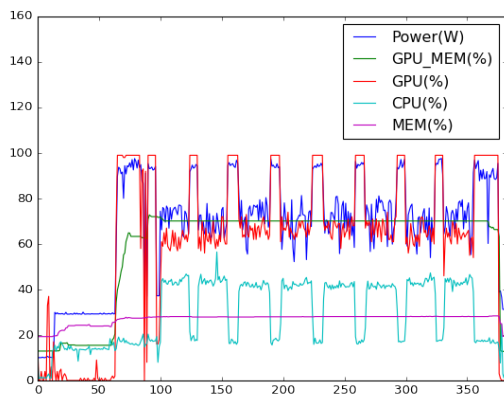
Figure 7: Profiling scene - high level profiling during scene playback created with nvidia-smi and Python psutil.
