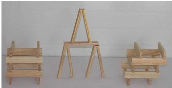
Figure 3: The three stack types, from left to right: 4-stack, card house and leaning tower.
