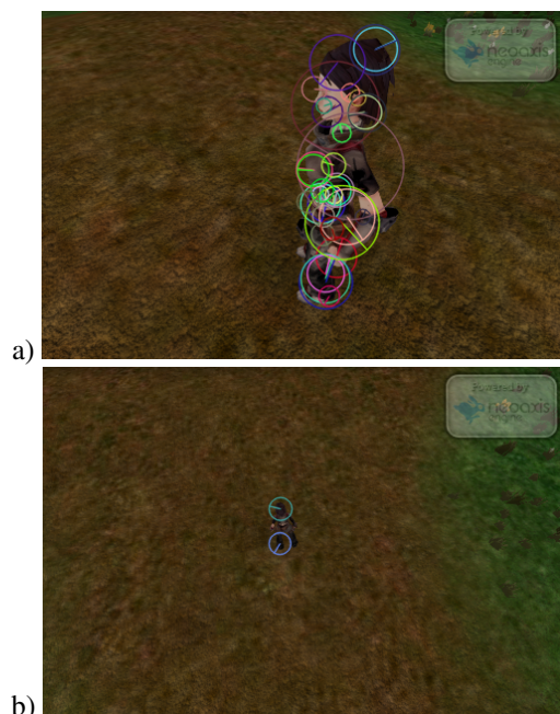
Figure 6: Key points identified within an object seen from the direction of 45^\circ (a) the Girl object seen from close distance, (b) the girl object seen from large distance
