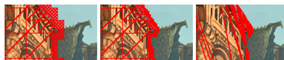
Figure 2: Sample triangulations generated with the Mip8, Mip2 and the contour-based methods. Images from [4].
