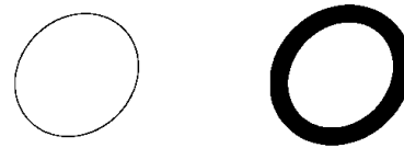
Figure 4: An elliptic band (on the right) is defined by the dilatation of a reference ellipse (on the left)
