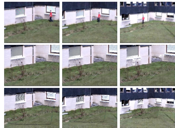
Figure 2: In the top row are 3 frames from the zoomIn-zoomOut video of the changedetection.net data set. The second row shows corresponding representations of the background model if the normal GSM is applied. There is almost no change in the background model although the camera zooms out because the model was trained already over a long time and adaptations now take a long time to happen. The last row shows the model with the addition of the proposed algorithm where the model adapts to the zooming motion.
