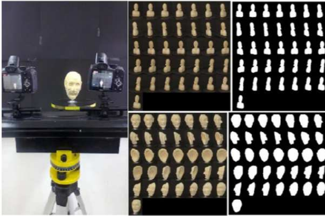
Figure 4: Real acquired sequence of archeological objects: 36 calibrated frames of "hannibal" and "punic mask" and their correspondent silhouette sequence.
