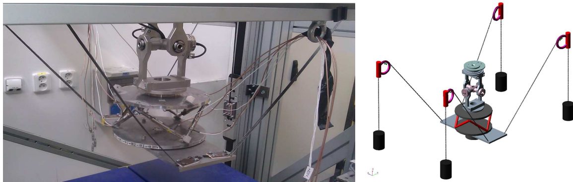
Figure 1: The QuadroSphere tilting mechanism and its visualization in the MSC.Adams software.
