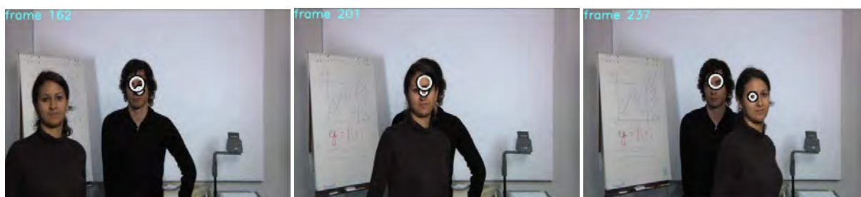
Figure 5: Tracking results of our method (big circle) and tracking results considering a single cue (small circles).
