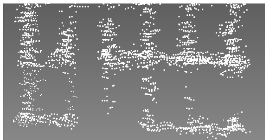
(a) Point cloud of reinforced bars
