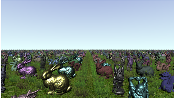
Figure 12: The virtual scene with two SDF components - one for Stanford objects and one for the grass objects. 24 FPS on Nvidia GeForce GTX 660, 100 FPS on Nvidia GeForce GTX 980.
