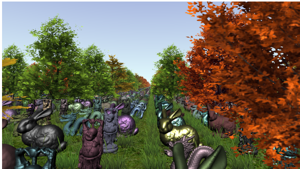
Figure 13: The virtual scene with three SDF components - one for Stanford objects, one for the grass and one for the trees. 32 FPS on Nvidia GeForce GTX 660, 93 FPS on Nvidia GeForce GTX 980.
