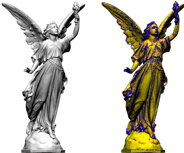
Figure 7: Estimated normal directions and curvature on the lucy model using the RMSE criterion. Point cloud is rendered using estimated normal directions (left), and curvature indicator (right).
