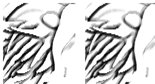
Figure 11: Ambient texture before (left) and after (right) the blur pass was applied. Note that the artifacts in form of single white pixels on the left image that disappear after the blur pass.
