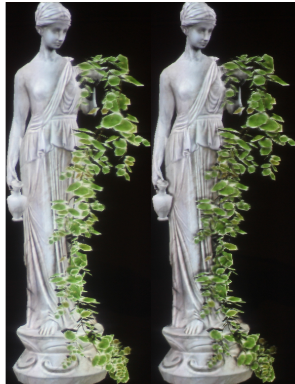
Figure 14: The model of statue rendered on the HoloVizio 640RC system 1 . Left image is rendered without SSAO effect, right image – with. Note that the images above are rendered with the help of multiple optical modules, not a single one. These images are not the same with the images for the optical modules from Figure 10.
