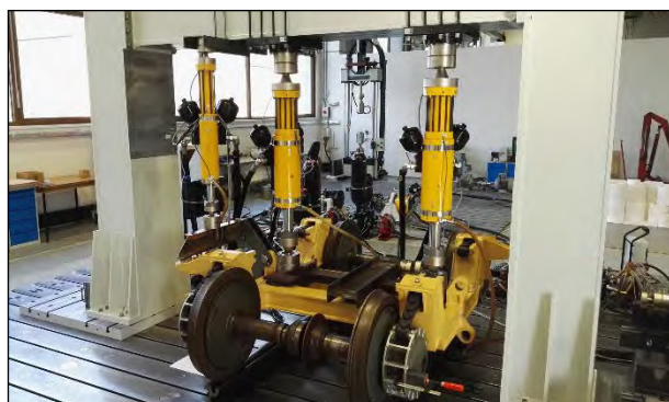
Fig. 3. Test of tram bogie with four actuators.
