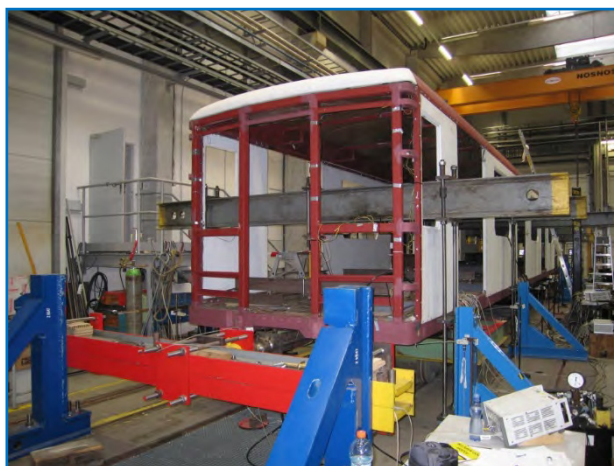
Fig. 6. Static strength test of hybrid body.
