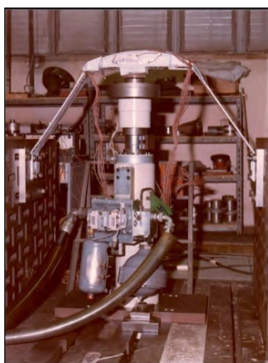
Fig. 14. Fatigue test of a front suspension holder.
