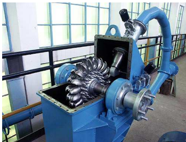
Figure 2.1: A Pelton turbine with the runner. (Source: [67])
