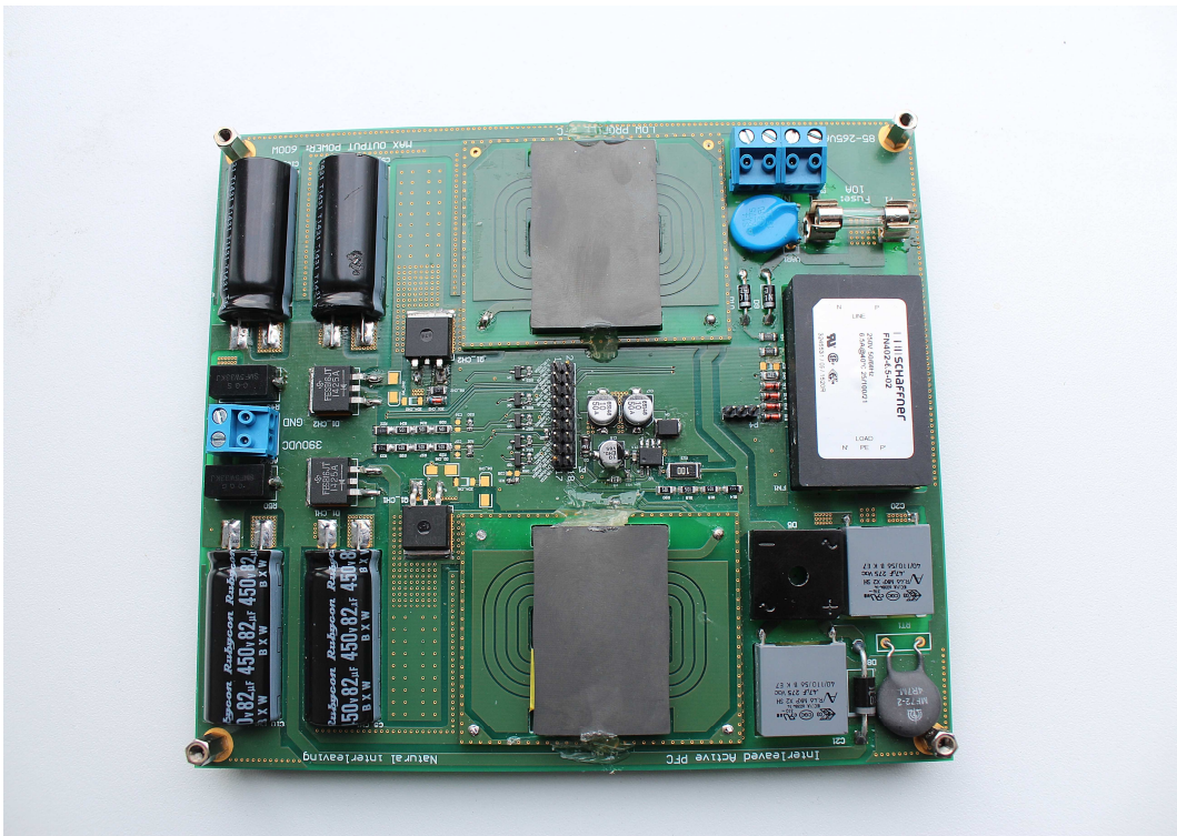
Fig. 8.12 Top view of the interleaved corrector.
