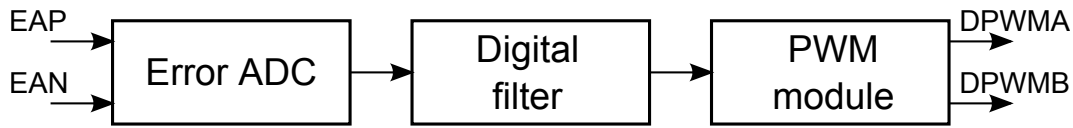
Fig. 10.7 Block diagram of the digital power peripherals.
