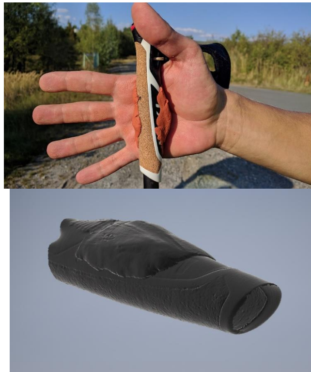
Figure 8: The memory foam and the 3D scan
