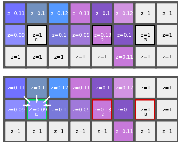
Figure 6: Fragment f1 is detected as a hole based on depth differences to its neighbors and gets assigned the minimum depth value within its neighborhood; f2 and f3 remain unchanged as they fail the distance threshold and the minimum number of neighbors, respectively.
