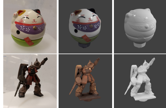
Figure 6: Reconstructed 3D models of speccat and hammerman. The real objects are shown on the left and rendered reconstructed outputs are shown on the middle and right.
