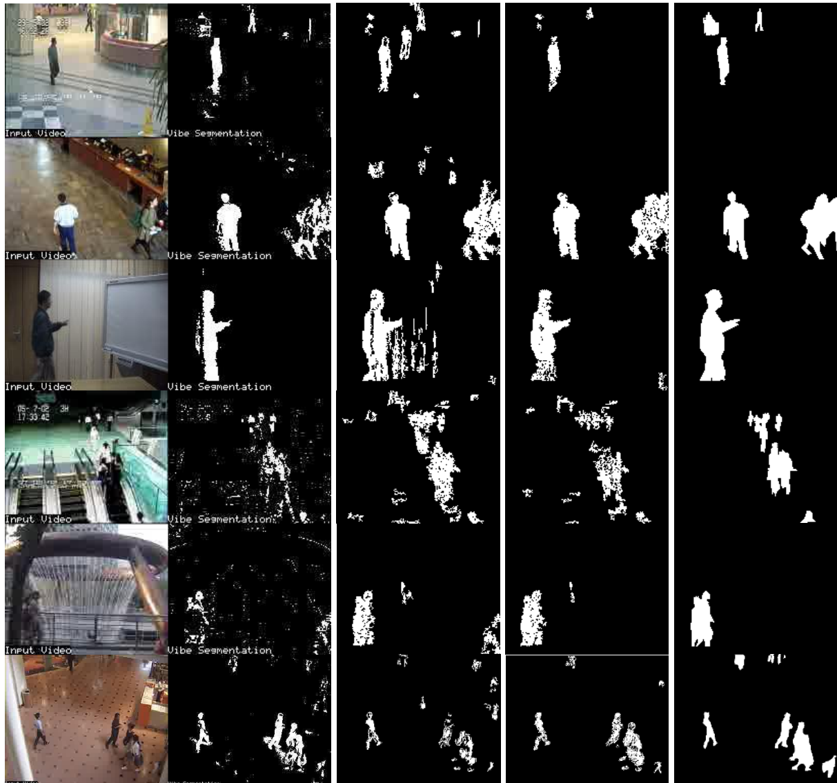
Figure 3. Background subtraction results on the Star dataset (9 image sequences) – original image frames (first column), results obtained by ViBe (second column), results obtained by MC-SILTP (third column), results obtained by our method (fourth column), ground truths (last column).
