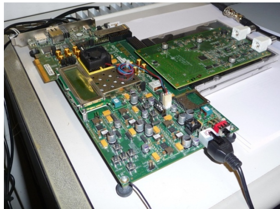
Figure 3. Analog front end plugged in the KC705 development board.
