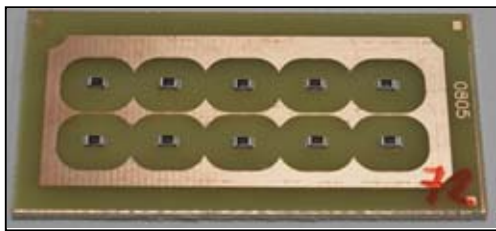
Figure 3. PCB with placed 0805 chip components.
