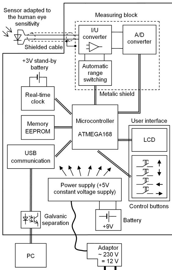
Figure 1. Block diagram of luxmeter connection.
