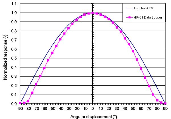
Figure 2. Measurement of the sensors' directional response patterns – horizontal axis of rotation.
