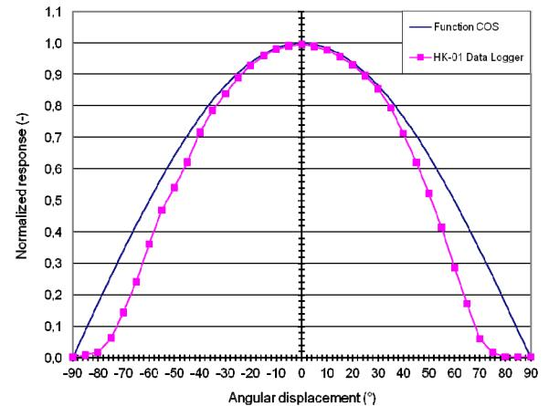
Figure 3. Measurement of the sensors' directional response patterns – vertical axis of rotation.
