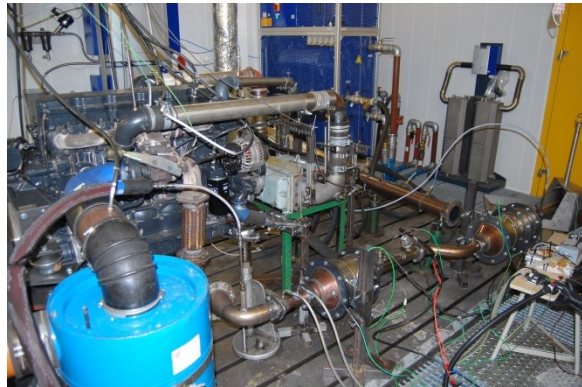
Figure 2. The engine test bench with the SCR system
