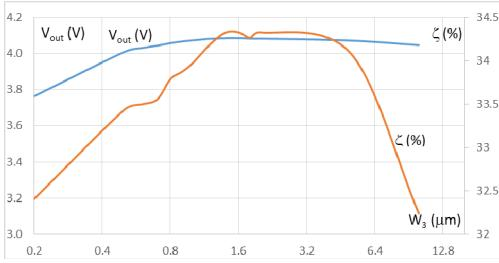
Figure 8. Variant 3: Efficiency and output voltage as functions of  $W_3$ .
