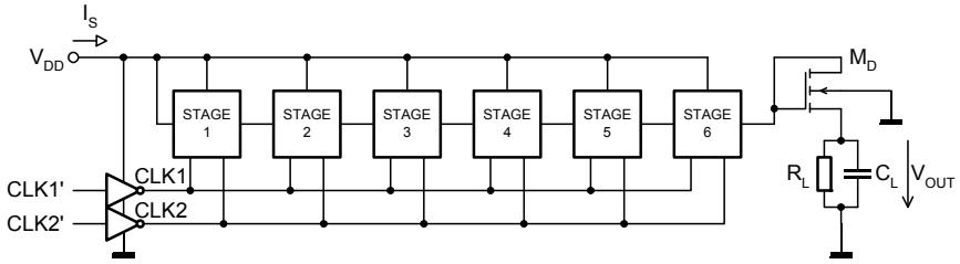
Figure 3. Simplified schematic diagram of simulated charge pump for  $N=6$ .
