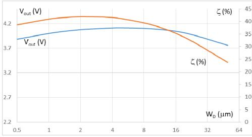
Figure 7. Variant 2: Efficiency and output voltage as functions of  $W_D$ .
