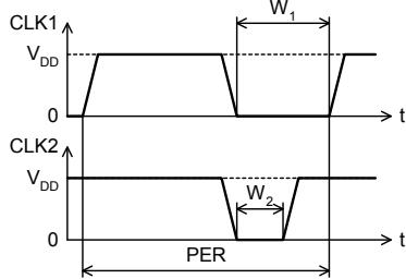
Figure 2. Waveforms of 2-phase clocks.
