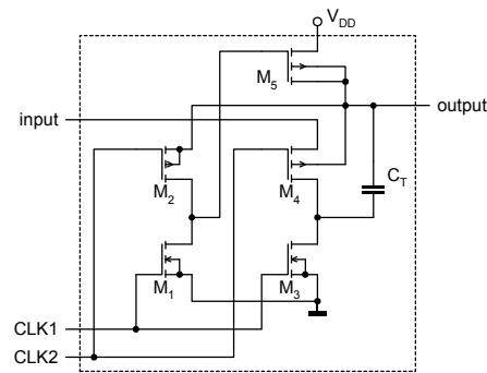
Figure 1. One cell of proposed charge pump [8].
