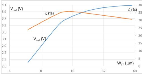
Figure 10. Variant 6: Efficiency and output voltage as functions of  $W_{CT}$ .
