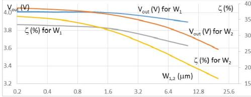
Figure 9. Variant 4, 5: Efficiency and output voltage as functions of  $W_{1,2}$ .
