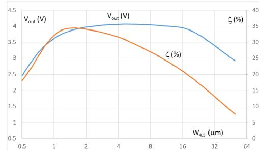
Figure 6. Variant 1: Efficiency and output voltage as functions of  $W_{4,5}$ .
