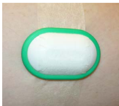
Figure 5 Temperature sensor fixated on skin
