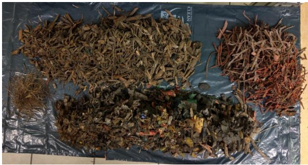
Fig. 2. Unwanted materials found in the ore.
