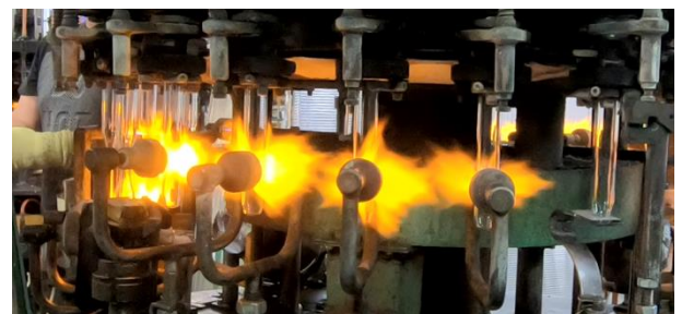
Fig. 2. Semi-automated process of blowing glass balls.
