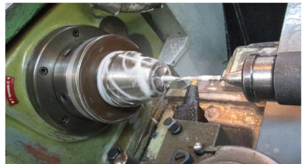
Fig. 2. Deep surface rolling processing on the surface of additively manufactured specimen.
