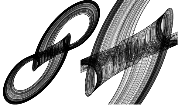
Figure 2. Three-dimensional view on strange attractor generated by first configuration of MVSM (left picture), detailed zoom on inner segment of a vector field (right plot).
