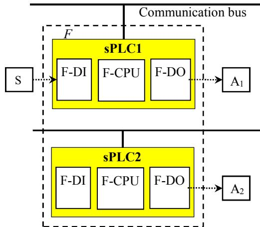
Figure 1. Safety function realised by simple decentralised SRCS
