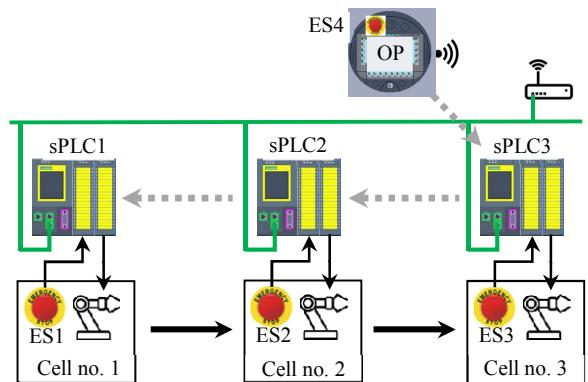
Figure 3. Production line with one-level decentralised SRCS
