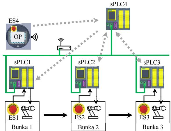
Figure 4. Production line and two-level decentralised SRCS
