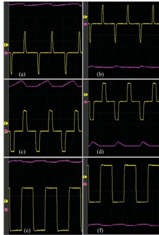
Figure 5. Oscilloscopes obtained for the steady-state response of V_{HV}^+ (a, c, e) and V_{HV}^- (b, d, f) for i_p and i_n pulses with 35 mA amplitude and 1 ms (a, b), 3 ms (c, d), and 10 ms (e, f) pulse-widths. Yellow waveforms represent i_{out} . Purple waveforms represent V_{HV}^+ (a, c, e) and V_{HV}^- (b, d, f). Voltage and time divisions are 20V/div and 10 ms for both channels.
