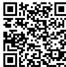
Fig. 1. Example of QR Code version 5, L error-correction level on alphanumeric mode.
