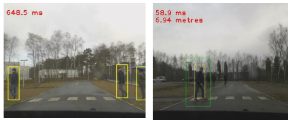
Figure 8. Pedestrian Detection with improved HOG/DPM approach under ESIGELEC Indoor/Outdoor dataset. Left top image: Pedestrian detection with calculated distance under DPM, Right top image: Pedestrian detection-based SSD deep learning model, Left bottom image: Pedestrian detection-based DPM, Right bottom image: Pedestrian detection-based Faster-DPM.
