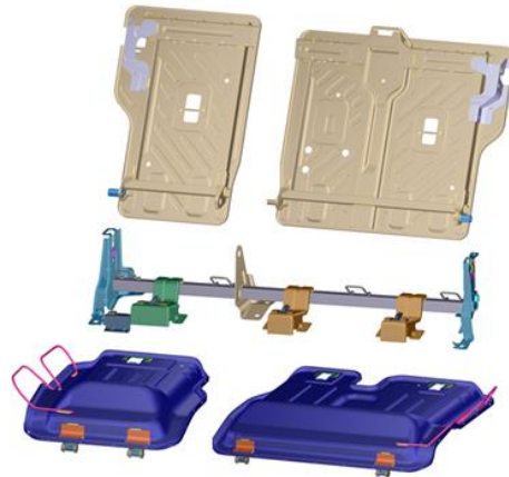
Figure 1 - Rear seat structure
