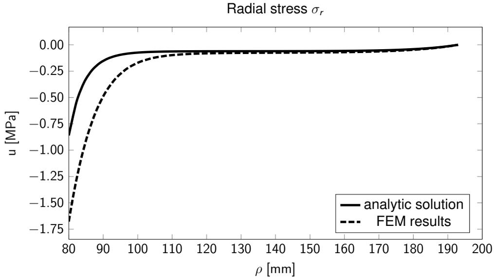
Figure 2. Difference between linear material and FEM solution using non-linear material
