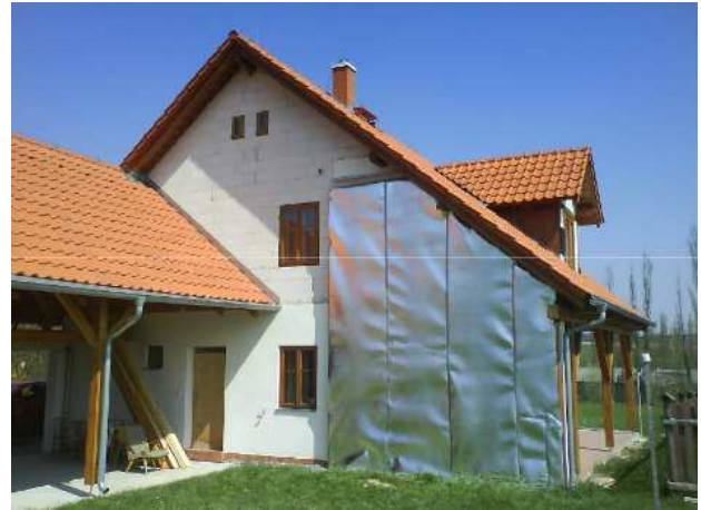
Fig. 5. Sensors calibration with reflective foil on trombe wall.
