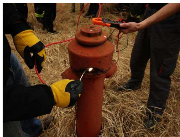
Fig. 9. Sample of secondary hazards – DC sparks.
