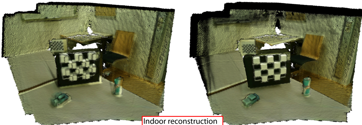
Figure 1: A partial room reconstruction using depth camera algorithms (e.g., InfiniTAMv3) is becoming increasingly popular. Simple reconstruction methods solely use the depth camera, leaving any imagery from the adjunct RGB camera untouched. Recent approaches also incorporate color camera information to improve consistency. However, the results heavily depend on the accuracy of the rig calibration, which can strongly vary in quality. Unfortunately, any errors in the rig calibration result in apparent visual discrepancies when it comes to colorization of the 3D reconstruction. We propose an easy approach to fix this issue for the purpose of image-based rendering. We show that a relatively simple warping function can be calculated from a 3D checkerboard pattern for a rig with poor calibration between cameras. The warping is applied to the RGB images online during reconstruction, leading to a significantly improved visual result.
