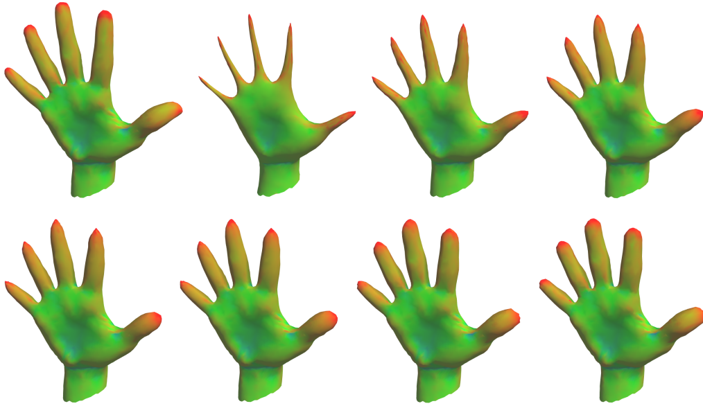
Figure 9.7: Influence of the power modifier n on a highly protruded model. Top to bottom, left to right: original model, simulation after 50 iterations with power modifier n = 1 , n = 2 , n = 3 , n = 4 , n = 5 , n = 10 and n = 20 . Using curvature color coding as described in Figure 9.1
