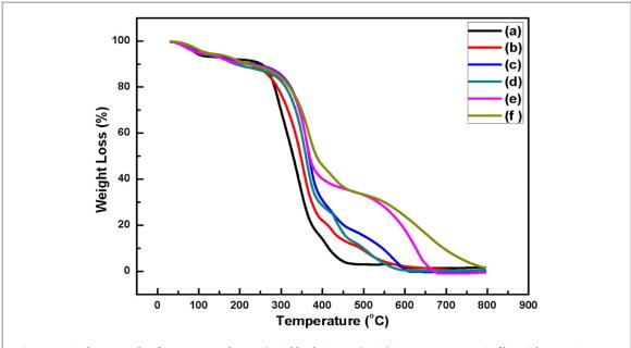
**Figure 3.** TGA thermographs of (a) Pure PVA, (b) PVA/PEG blend, (c) PVA/PEG/CBNPs nanocomposite films with 5 wt% CBNPs, (d) 10 wt% CBNPs, (e) 15 wt% CBNPs, (f) 20 wt% CBNPs, (g) 25 wt% CBNPs.
