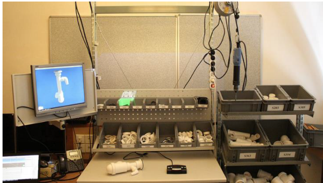
FIGURE 2. Workplace designed for the experiment, in configuration for group 3DIO (3D animated manual, in-situ marked box, special controller).
